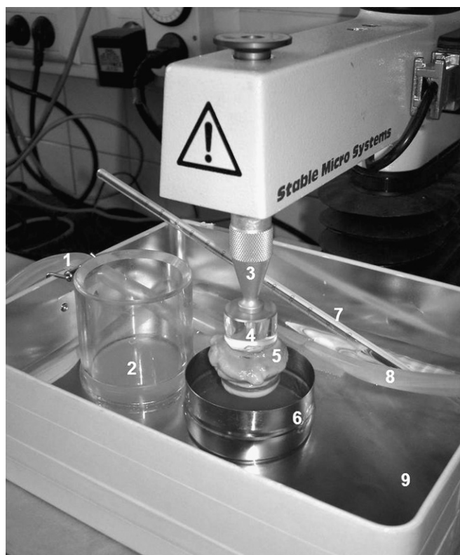
Fig. 1. Mucoadhesion testing apparatus. 1 – water in; 2 – immersion fluid; 3 – probe holder; 4 – probe; 5 – mucosa; 6 – sample bottle; 7 – thermometer; 8 – water out; 9 – water bath.
